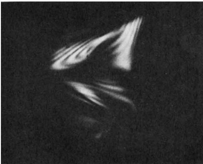
Fig. 13. Isochromatic (top) and 80° isoclinic (bottom) patterns for PVF 2 at 210°C and q = 0.02 \text{ cm}^2/\text{s} .
